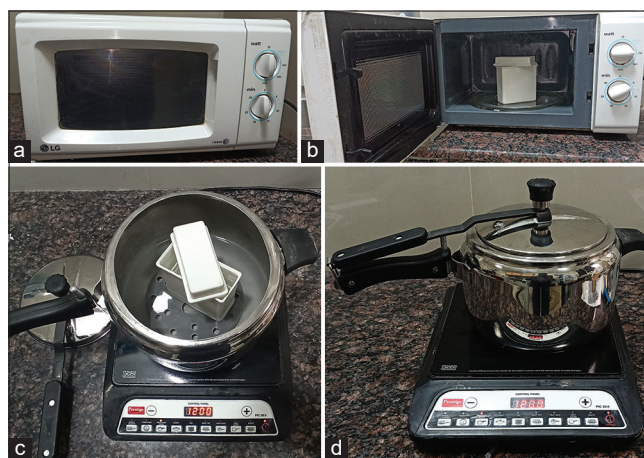
Figure 1: (a and b) Microwave oven antigen retrieval method. (c and d) Pressure cooker antigen retrieval method.
